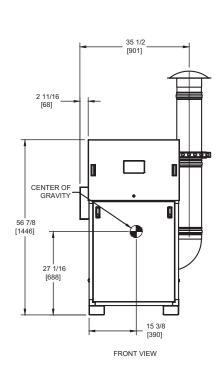
29<sup>°</sup>1/2 [749] TOP VIEW 77 1/16 [1957] 68 15/16 [1750] 45 [1143] 1 1/2 [38] CENTER OF GRAVITY 000000 30 11/16 [25] [780] 66 1/2 [1689] 1 3/8 [36] SIDE VIEW 4X 3/4 [19] 2 1/2 [64] 4X .438 [11] 12 5/16 [313] 1 24 [610] 12 5/16 [313] BOTTOM VIEW
